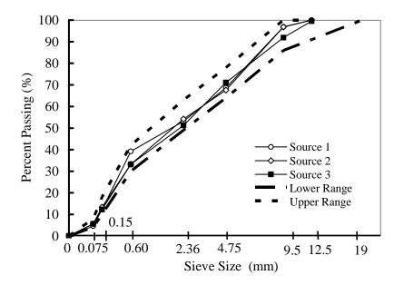
Fig. 1 Gradation curves for Sources 1, 2, and 3 (SCDOT Type I surface source)
