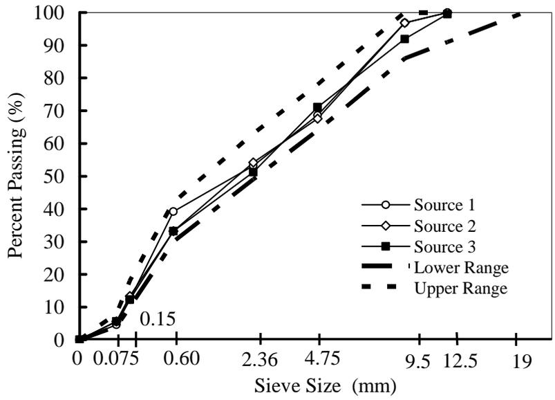
Fig. 1 Gradation curves for Sources 1, 2, and 3 (SCDOT Type I surface source)
